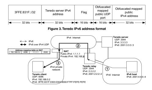
Figure 4. Communication between a Teredo client and an IPv6 host
