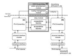
Figure 6. Architecture of NICI-Teredo relay
