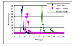
Figure 8. Encapsulation latency histograms of Teredo relay (1280 bytes) Formatted: Bullets and Numbering
