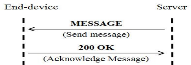
Figure 7. Signal flow of instant messages
